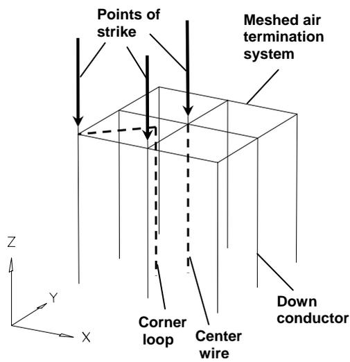
b) Structure dimensions: Length 20 m, width 20 m, height 20m
