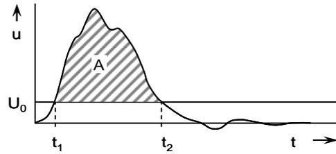
Fig. 5. Illustration of the constant-area-criterion
