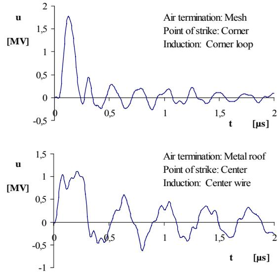
Fig. 4. Examples of induced voltage waveshapes
