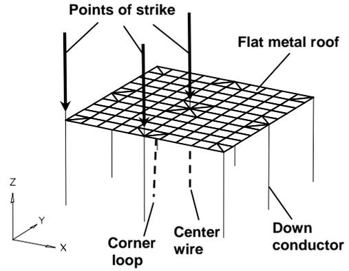
a) Structure dimensions: Length 20 m, width 20 m, height 10m
