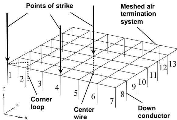
c) Structure dimensions: Length 60 m, width 60 m, height 10 m
