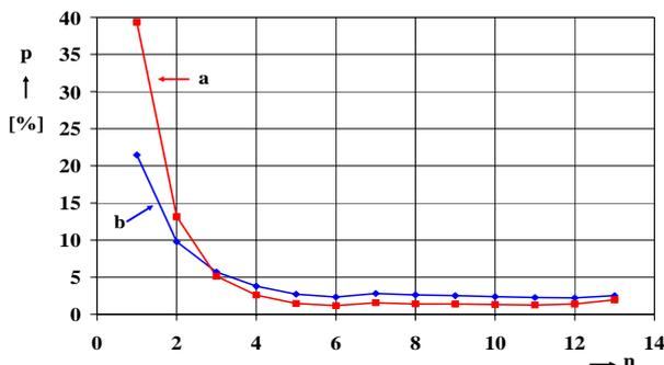
Fig. 3. Percentage current distribution to the down conductors for the 60 m x 60 m x 10 m structure, lightning strike to the roof corner
