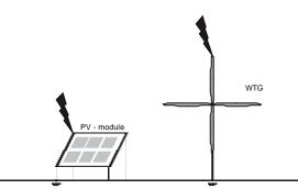
Fig. 4: Integrated LPS with direct strikes to the components (here: PV-module and small WTG).
