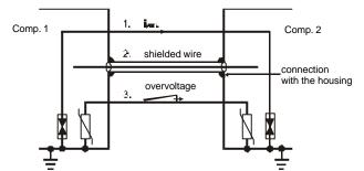
Fig. 6: General measures for the overvoltage protection.
