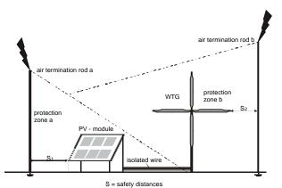
**Fig. 5**: Isolated LPS preventing the components from direct strikes (here: PV-module and small WTG).
