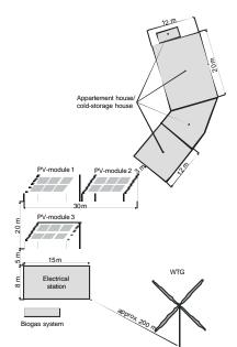
Fig. 3: Arrangement of VATALI's main parts.
