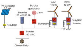
Fig. 2: Schematic diagram of the hybrid-system VATALI (extract).
