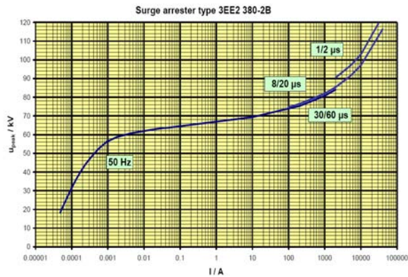
Figure 1: Characteristic curve of a 27 kV-surge arrester.
