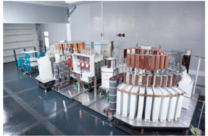
Fig. 9. Tandem pulse generator for lightning current up to 400 kA, 10/350 \mu s
